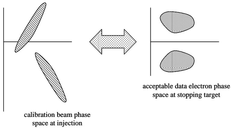
A schematic representation of phase space mapping between data electron coordinates (in the vicinity of the stopping targets) and calibration electrons at injection.
