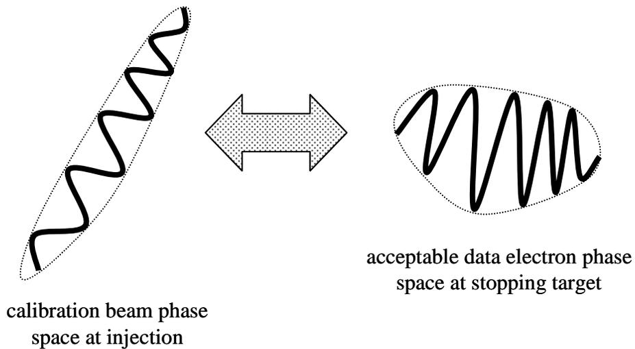
Phase space mapping between data electron coordinates and calibration electrons at injection when the calibration samples, rather than painting the full phase space.
