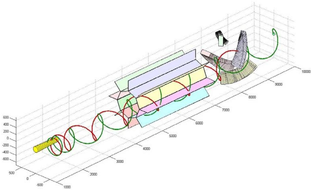
Downstream injection of a 105 MeV/c calibration electron.
