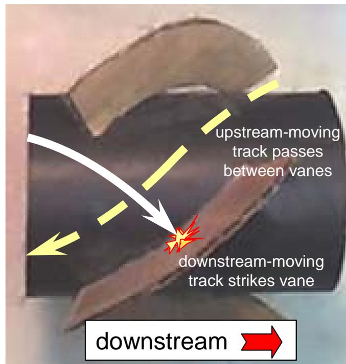
Downstream-moving (solid) and upstream-moving (dashed) electron trajectories. Note how the dashed trajectory threads its way between calorimeter vanes without interference while the solid trajectory strikes a calorimeter vane.
