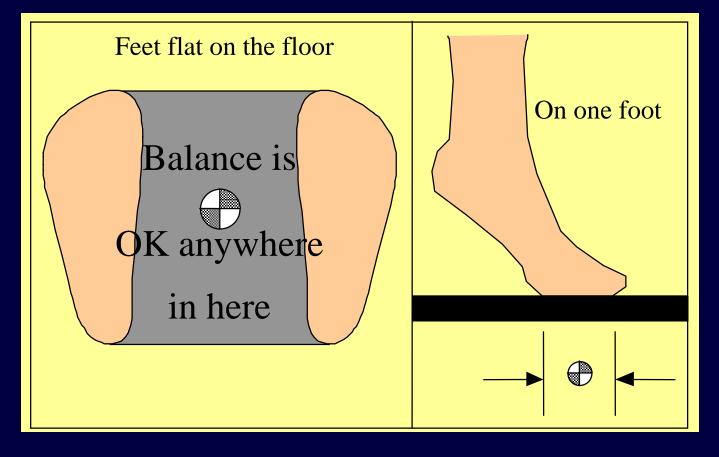
Staying balanced: center of gravity remains directly above the area of contact with the floor. (Otherwise  $\vec{\tau} \neq 0$ : you'd tip over.)
