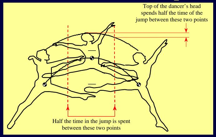
Half the duration of the jump is spent between the points indicated by the arrows; the height of the dancer's center of gravity only changes by 6 inches during this time.
