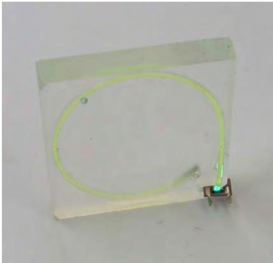
Fig. 2: Example of a SiPM mounted in the scintillator as in an HCAL tile.
