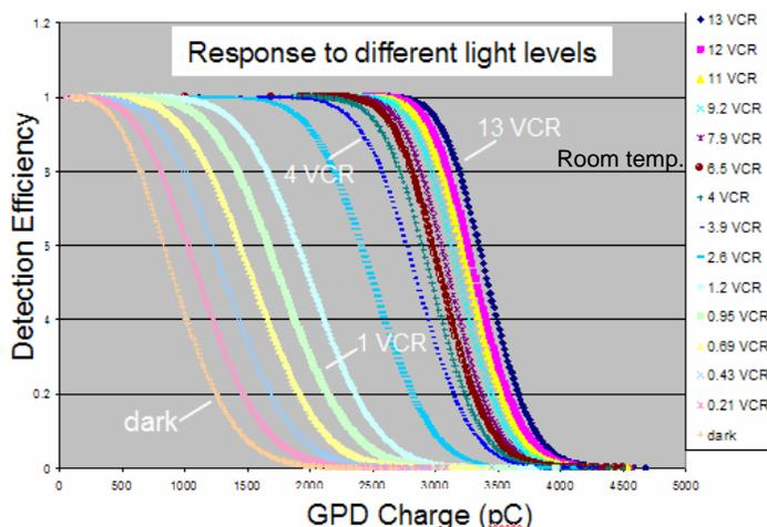
Fig. 4: Detection efficiency of a pixel as a function of the measured charged for a range of incident intensities.
