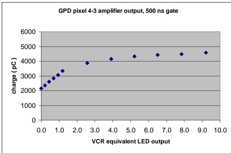
Fig. 3: GPD response (peak of the charge) distribution as a function of LED light intensity equivalent to the light yield from a MINOS bar.
