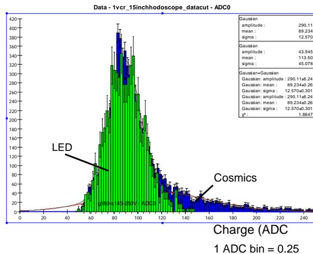
Fig. 2: Matching pmt response to cosmic rays in a MINOS bar to 550 nm LED pulses.
