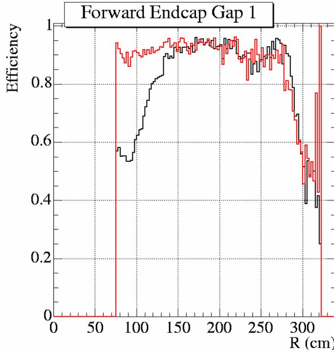
Fig.4. RPC efficiency as a function of R when the middle east chamber of layer 1 was operating in streamer mode (black) and in saturated avalanche mode (red).
