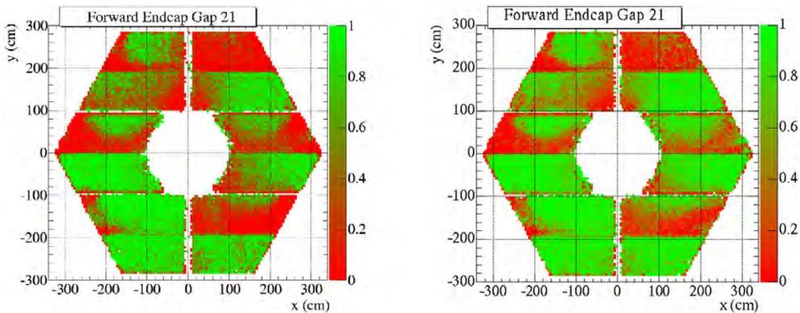
Figure 3. Two-dimensional efficiency of Layer 16 before and after 3 months of humidified gas.
