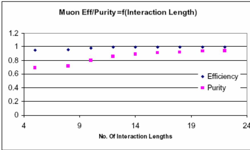
Fig. 1. Muon efficiency and purity versus the number of interaction lengths of the hadron calorimeter plus muon system for a muon identification algorithm developed by C. Milestene of Fermilab. The muon purity increases from 69% if only the calorimeter information is used ( $4.2 \lambda$ ) to 94% (if most of the coil and muon steel is penetrated) in a sample of  $bb$  jets @  $500\text{GeV}/c^2$ .
