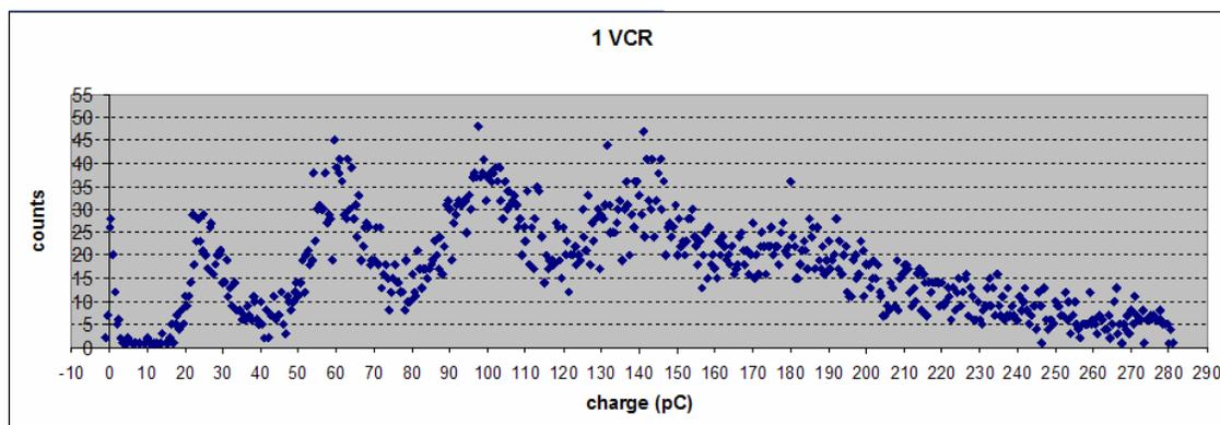
Figure 5: Demonstration single photon resolution for 1 vertical cosmic ray equivalent LED output at  $-19^{\circ}\text{C}$ . The peaks correspond to 1, 2, 3, 4, etc. photoelectrons.
