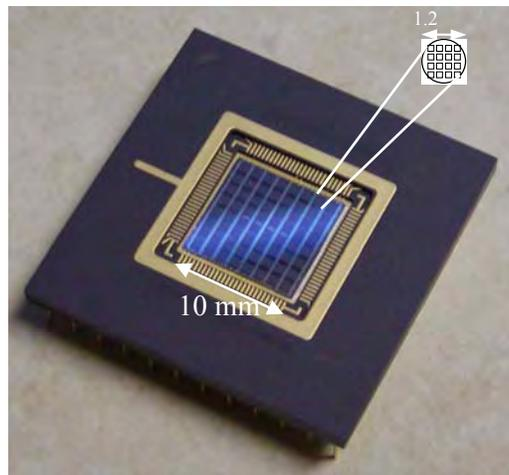
Fig. 1: 64-fiber readout prototype device produced by aPeak Inc.
