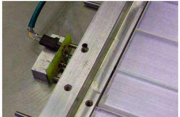
Fig. 3: Example of a SiPM mounted close to the scintillator as for the muon detector.
