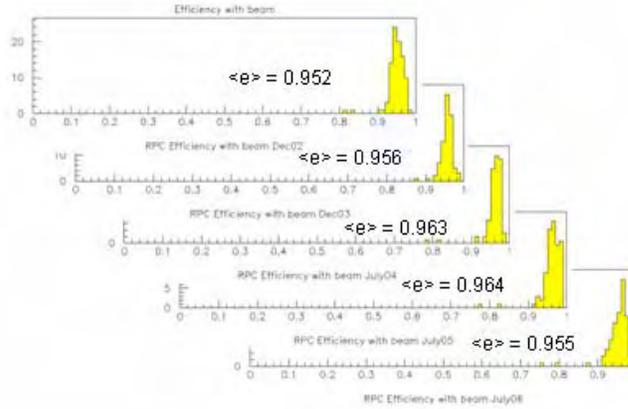
Fig. 2. Efficiencies of BaBar RPCs in positions with the lowest backgrounds at Dec. 2002, Dec. 2003, July 2004, July 2005, and July 2006 measured by  $\mu$  pairs in data.
