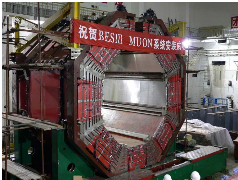
Figure 1. Installed BESIII barrel muon detector.
