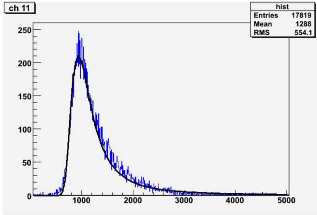
Figure 5: Pulse height distribution from a 120 GeV proton beam
