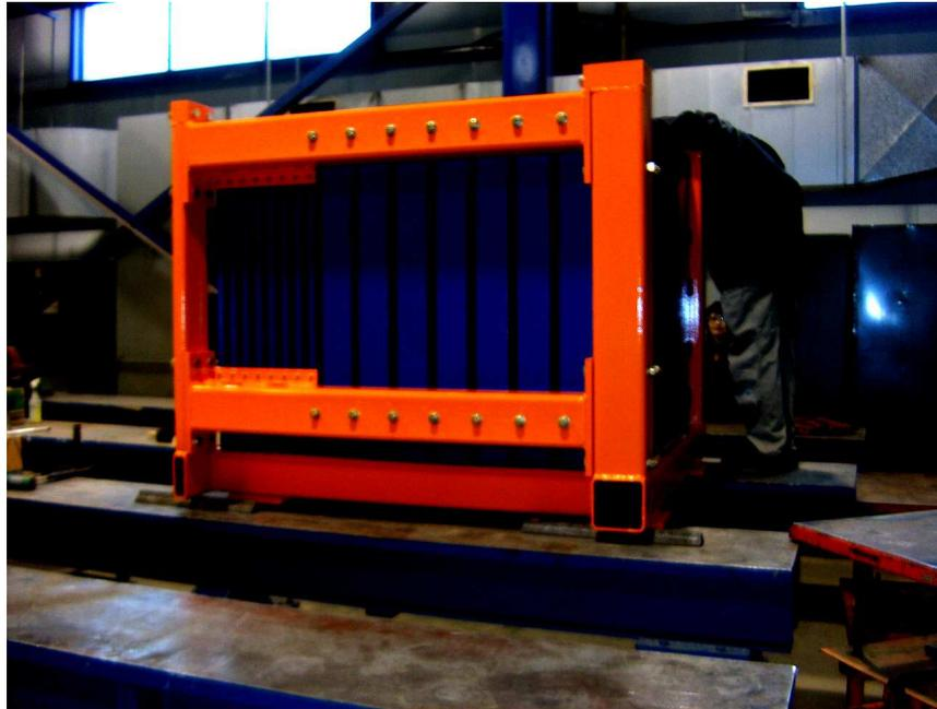
Figure 6: TCMT absorber stack structure.
