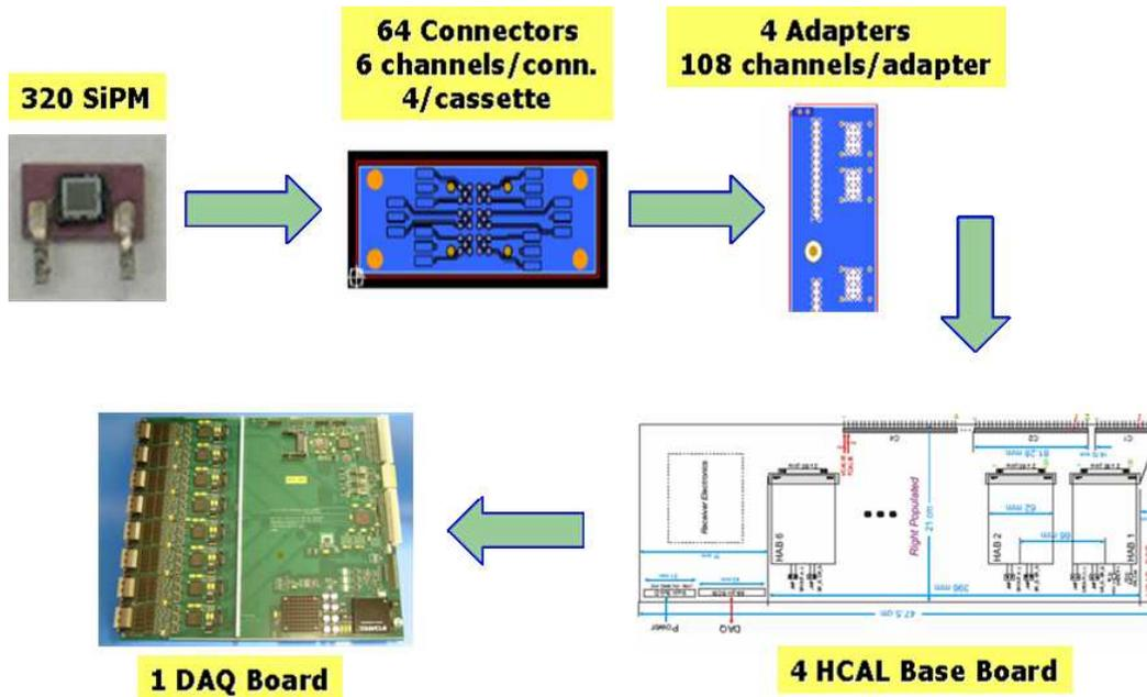
Figure 3: Electronics architecture for the TCMT.
