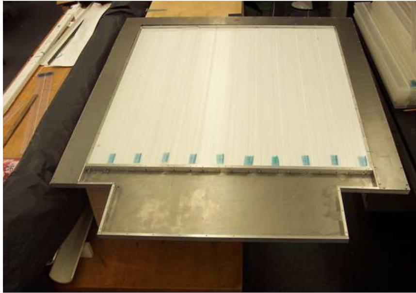
Figure 2: Mechanical prototype of cassette.
