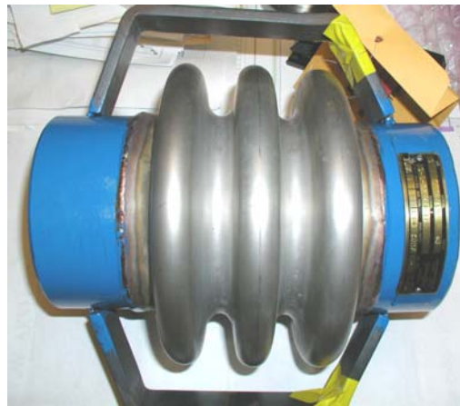
Figure 3. Hydro-formed stainless steel bellows, 2.75" minor radius, 4.25 " major radius.
