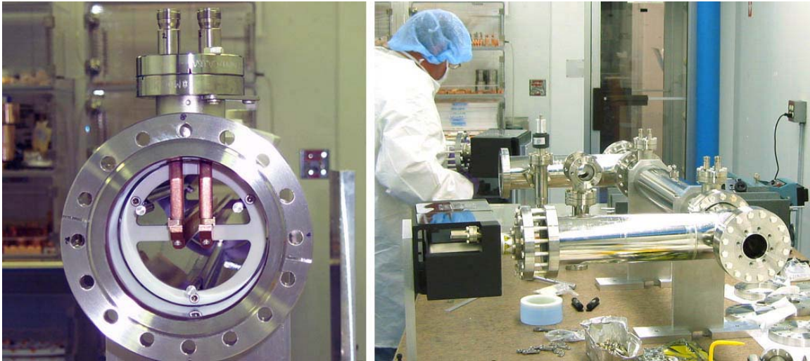
Figure 1. Kicker assembly. Left photo: electrodes, visible inside the vacuum vessel. Right photo: installing ion pumps.
