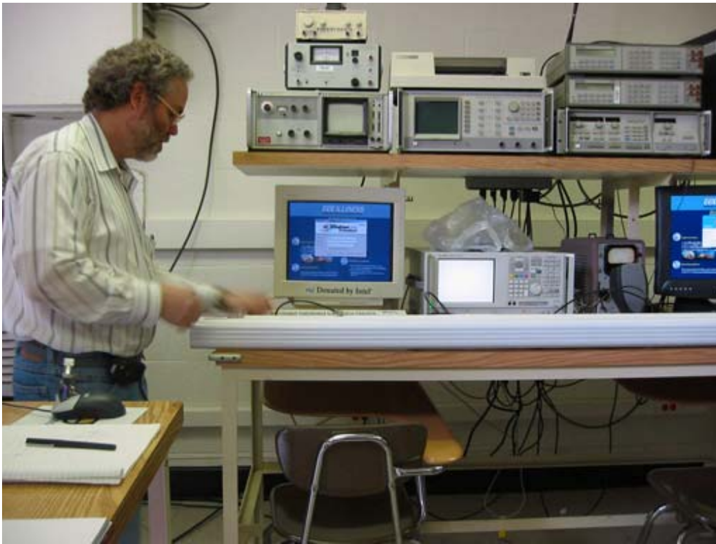
Figure 10: Preparation for measurements of the RF properties of 4"×3" aluminum downspout used as L-band waveguide. The dimensions should correspond to a cutoff frequency f_{cutoff} = 1.47 GHz.
