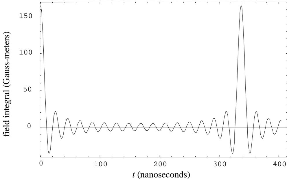
Figure 1. Field integral (Gauss-meters) vs. time (ns) in a 17-element system. Bunches 1 and 34 are kicked, while damping ring bunches 2 through 33 pass through the kicker during the zeroes of the field integral.
