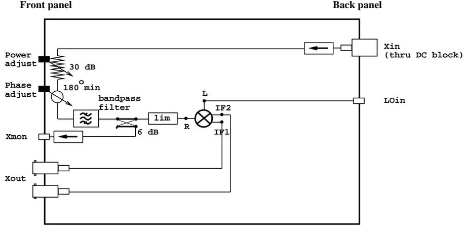
Figure 1: Schematics of the custom BPM signal processor.
