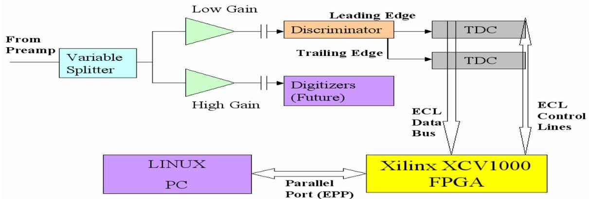
**Figure 4:** A box-diagram of the readout system that was developed at UCD for use at the prototype muon detector test-stand at Fermilab.
